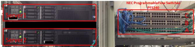
Fig. 5. The testbed used in our prototype evaluation. Our testbed is composed by two servers HP DL380G7 equipped with two Intel L5640 (6-Core 2.26GHz) processors, 24GB of RDIMM PC3-10600R-9 memory and by three NEC ProgrammableFlow PF5240 OpenFlow-enabled switches.
